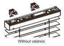
Choose one of below ways to attach the headrail to bracket. Start with attaching the headrail front to the bracket first.
